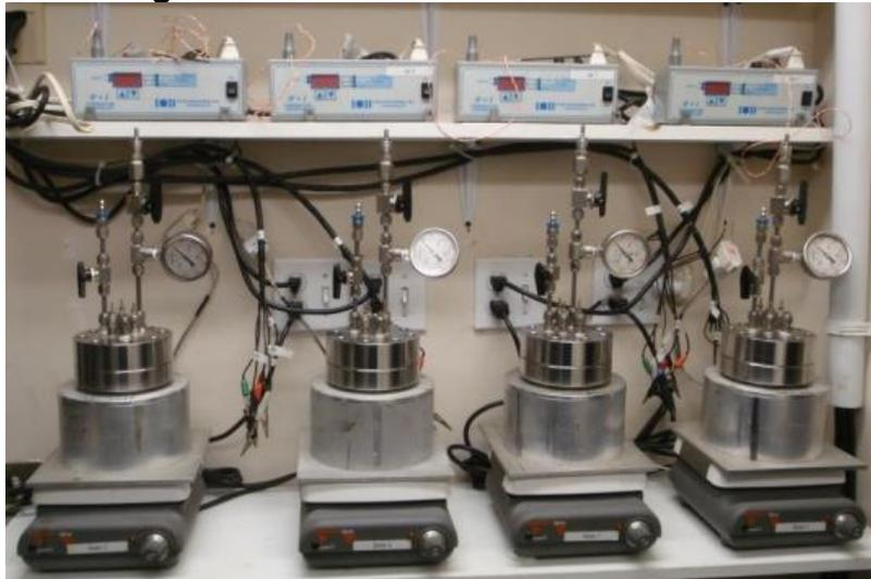
Figure 2: Photograph Showing the Autoclaves
