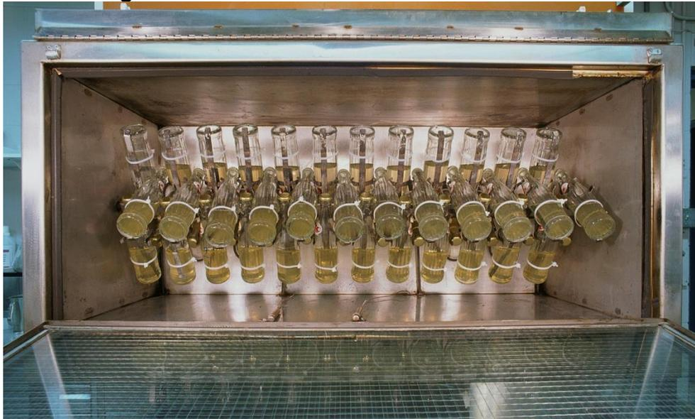
Figure 3 Photograph Showing Wheel Test Apparatus
