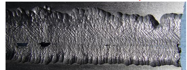
Failure line at ERW (11:00)
